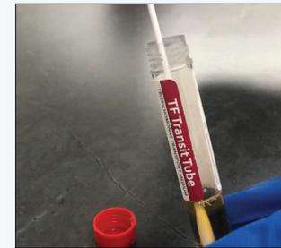
Insert the sample into the transit tube (0.5-1.0 mL of specimen). Secure the cap on to the transit tube and store it away from light. Ensure to record sample-related information on the label.
